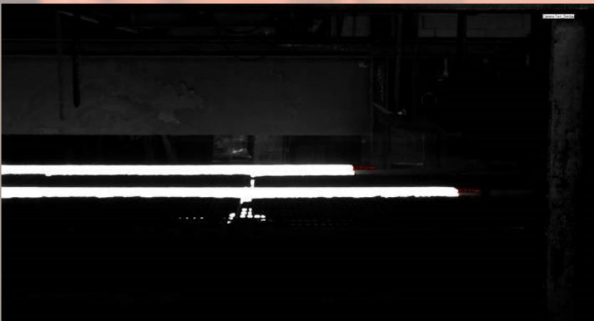
Processed Image, Billet row 3 & 4 running. Notice software reading billet length as it moves from the left to right on screen.
