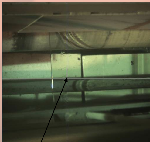
Inner Knurl Edge Tracked by CautyVision™ (note cross-hair position)
