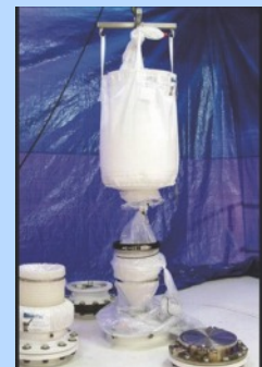
Vessel Charging and Sampling with Dover Pac®
