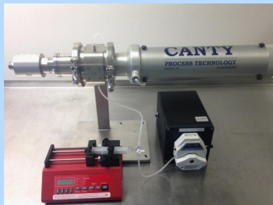
Automated syringe pump feed mechanism & dilution pump
