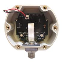
With the gauge powered up, press and hold the UP button. Release the button when the engineering units begin to flash.
