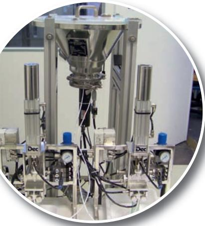
Dec now offers a much-anticipated solution in the volumetric dosing of small quantities of powder. The product is filled in a calibrated chamber of variable volume by action of vacuum and emptied either mechanically by a piston or by applying pressure.
