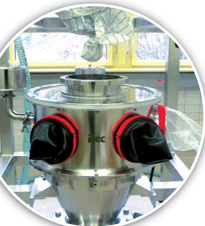
DCS Connection Head for high containment
