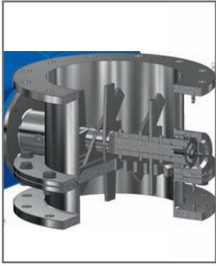
The device consists of a solid cylindrical body with inlet and outlet flanges, an integrated crushing tool which is driven by a laterally located motor and a grid. To obtain the required size, the blades and the grid are easily removable and can be adapted according to product characteristics.
