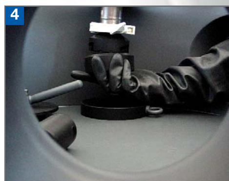
4 Removal of the suction lance protection cover before introducing the suction lance into the drum
