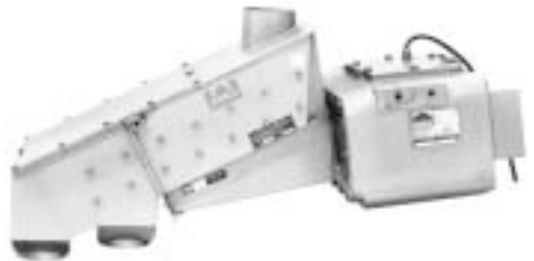
Model 70B Vibratory Sand Classifier used in conjunction with wood-fired boiler, to reclaim unburned wood for recirculation through boiler. Screens are used to sift out ash and sand.
