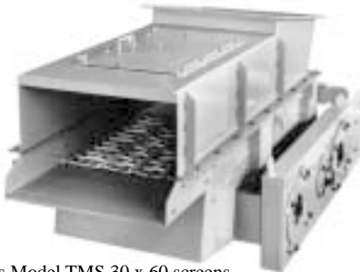
This Model TMS 30 x 60 screens oversize clumps of ore.
