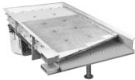
A two-deck screening feeder discharges oversize and undersize products to one side while the desired material flows off the end.
