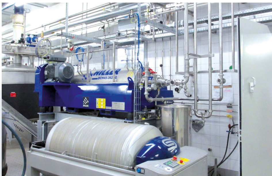
Hiller decanter in a chemical process
