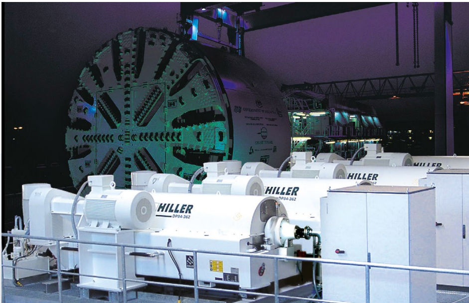
Hiller decanters in tunnel construction
