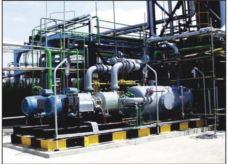
Duplex vacuum system used on a crude oil distillation tower
