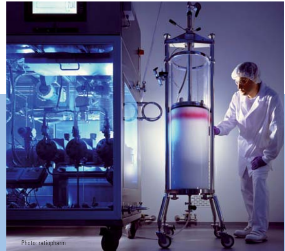
By intelligently overlaying the feed flows of two single pumps, it is possible to prevent pressure pulsation, even without pulsation dampers.
