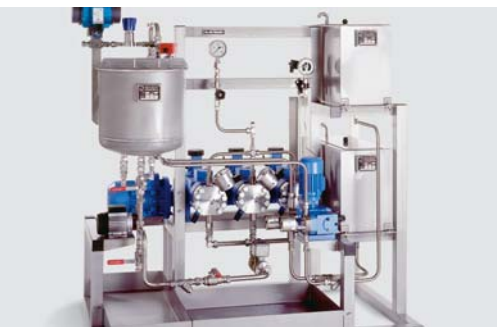
Precise and reproducible: fully automatic compact package for recipe controlled production of dispersion adhesives
