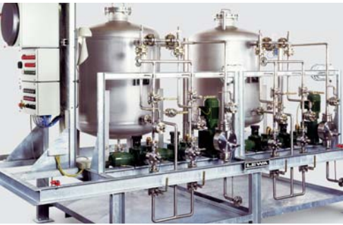
Precise and continuous: metering- and mixing packages for the production of fabric softeners
