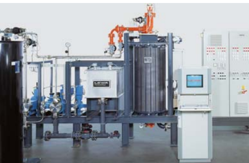
Different concentrations: metering- and mixing packages e. g. for acid dilution
