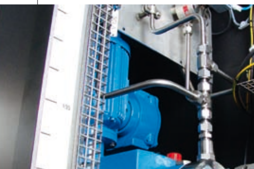
Sight glass for fill level indicator and pump calibration
