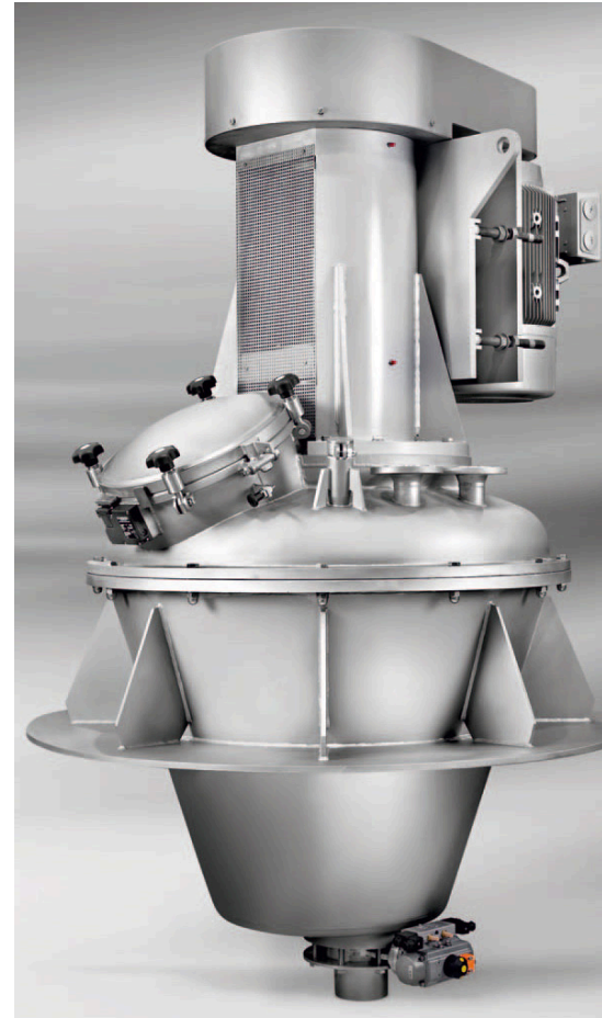
Wet Mixer type NOHK mainly used for the production of baby food
