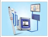
Provides greater process reliability with real-time sensor aging monitoring through ISM technology via HART.
