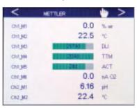
A configurable display allows the highest flexibility to view the most important values. The Wizard set-up allows the definition of favorites to directly reach any menu.
