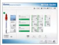
With iSense<sup>™</sup> software, sensors can be calibrated via a PC or mobile device then connected to the M100 DR. Therefore, a user interface in the field is not necessary.
