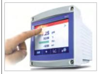
Touchscreen display provides simple, convenient operation, and any menu function can be reached in only three touches. Traffic light color coding means process or sensor issues are visible from a distance.
