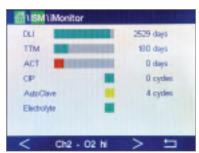
With its unique iMonitor diagnostics utility, the M800 predicts sensor maintenance and details corrective actions – before issues arise.
