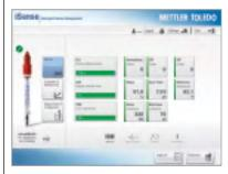
With iSense<sup>™</sup>, the key tool of ISM, sensors can be precalibrated via a PC then connected to the M100. Therefore, a user interface in the field is no longer necessary. This new transmitter concept reduces the operation and wiring effort to a minimum.
