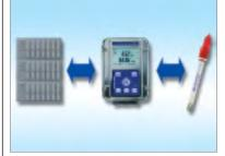
M700 transmitters with ISM technology allow seamless integration of online sensor diagnostics into process control systems over PROFIBUS PA and FOUNDATION fieldbus.
