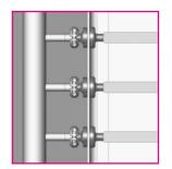
Vacuum tight feedthroughs for the connection nozzle of the heated inserts in the backwall of the vacuum chamber. The inserts and the distributor tube for the heating media are removable.
