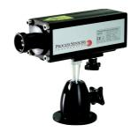
The detector is sensitive to infrared radiation in an area called the "cone of vision". Refer to Chart 1 for the spot size diameter at the shortest, midrange and longest variable focus distances. The cone vision/aperture diameter at the optical lens is about 16 mm. This area has to be kept free from any intervening objects. The spot size diameter for distances not given in the chart can be calculated by interpolation.
