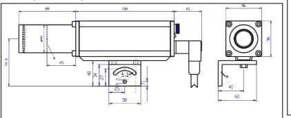
**Notice:** A variety of standard mounting, cooling, purging, IR window accessories etc. are available upon request.
