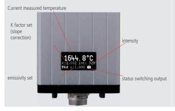
The parameters can be adjusted with the keys at the rear side of the device. The set value is taken over directly.
