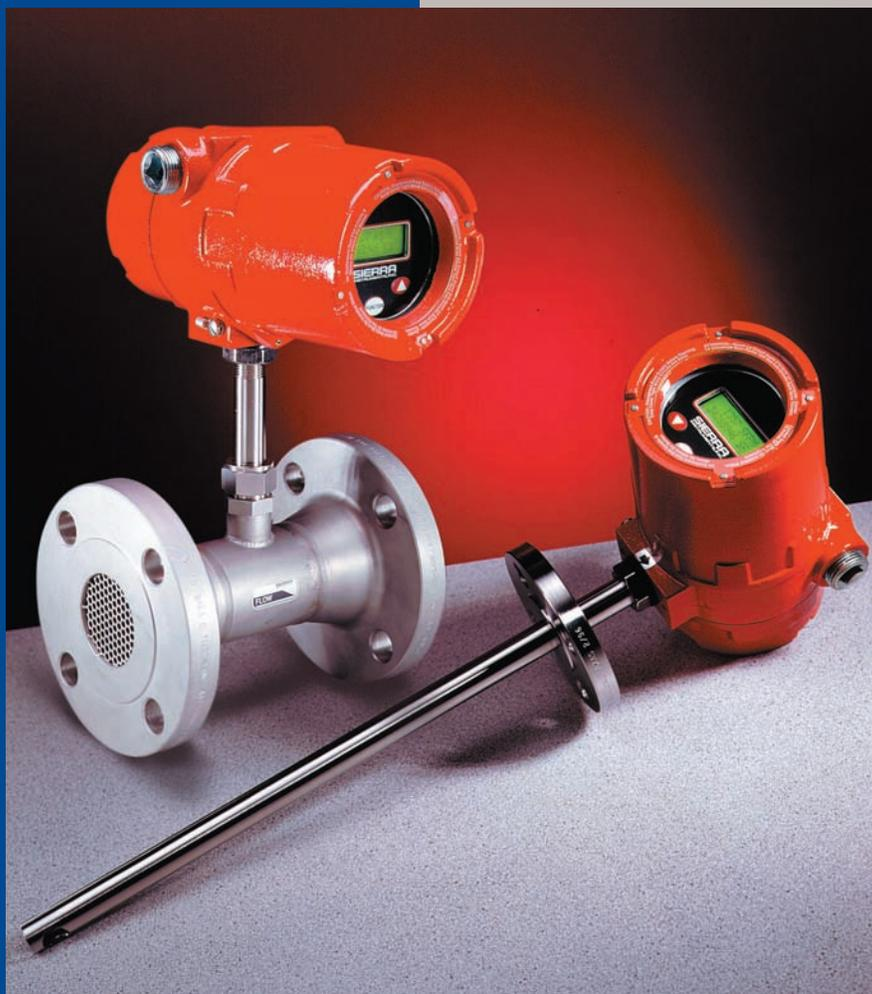
Mass flow rate and totalized flow, as well as other configuration variables, are displayed on the meter's optional 2 x 12 backlit LCD panel. The programmable transmitter is easily configured via an RS-232 serial port and Sierra's Smart Interface PC-based software; or via the display and function switches on the front panel of the device.
