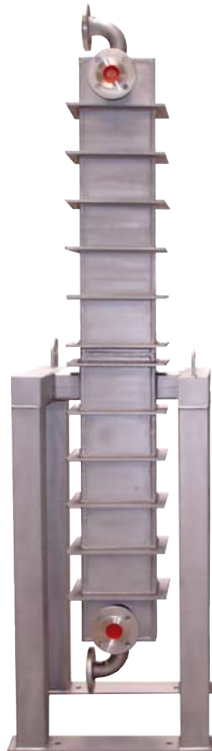
Fully-welded OPW-42 with reinforced ribbing. Two-pass design in full Stainless Steel 316L construction.
