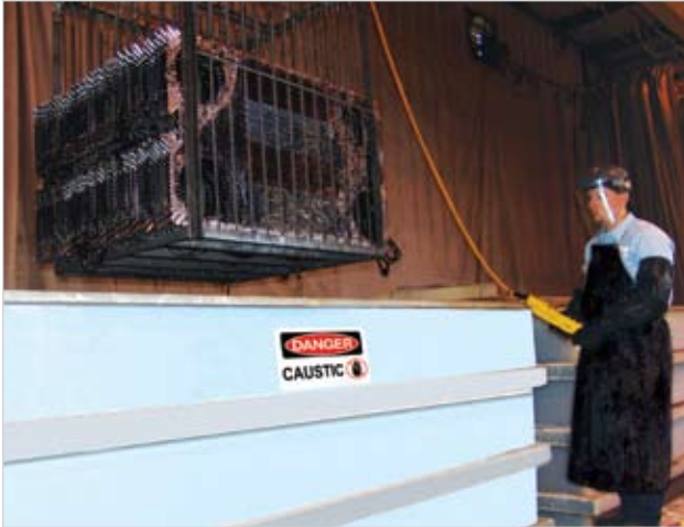
Plates are immersed in caustic and acid baths compatible with the plate material.
