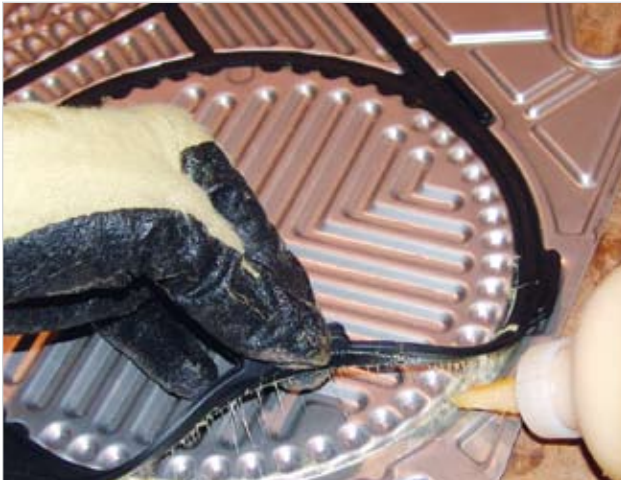
Plates are regasketed with OEM replacement gaskets, using a non-hardening, OEM-spec adhesive that does not require heat curing.
