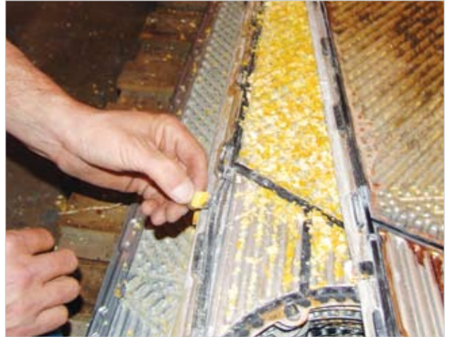
Plates and gaskets from other manufacturers are analyzed to determine if original specs still apply, and what cleaning procedures will be most effective.
