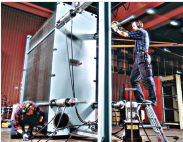
Entire unit refurbishment includes frame repair, complete plate pack service, reassembly and closing the unit to precise factory specifications.
