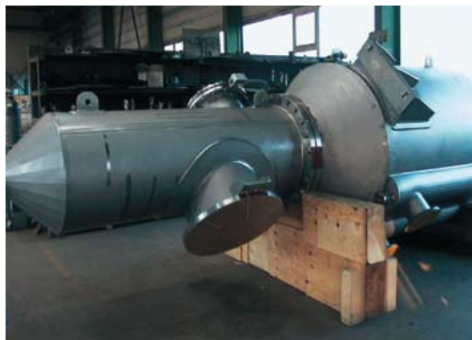
Spiral HE configured as a bottom condenser.
